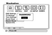
To reset the receiver to factory default settings, select Master Reset and press OK. A PASSWORD window will appear. Using 0-9 keys enter your password and the WARNING message will appear. Press OK to reset or EXIT to abandon resetting.
